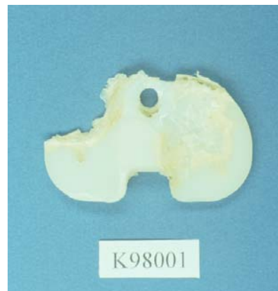
Worn UHMWPE component of total knee replacement.
