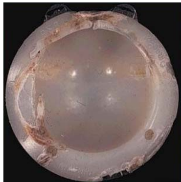
Worn UHMWPE cup of total hip replacement.
