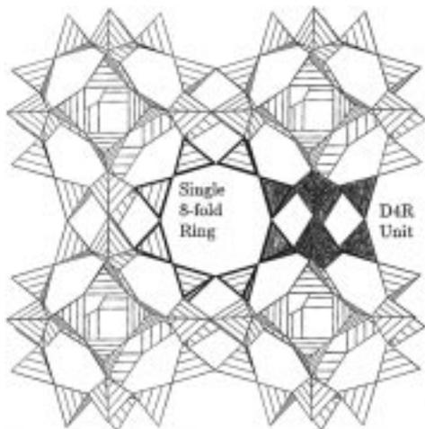
**Figure 6.** Framework structure of zeolite LTA. The shaded region is a D4R unit, and these form the connections between the sodalite cages. The heavily outlined tetrahedra form a single 8-fold ring (S8R). Note that every tetrahedron is simultaneously part of a D4R and a S8R.
