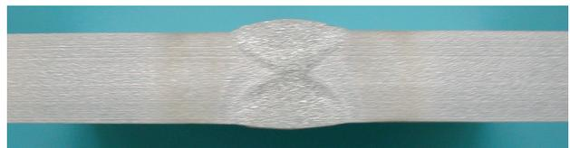
Figure 1. Macrograph of weld cross-section showing the double-V shape of the weld. The weld was fabricated in two passes, on either side of the plate.
