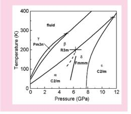
Figure 1. Pressure-temperature phase diagram of solid oxygen at P<12 GPa [2].
