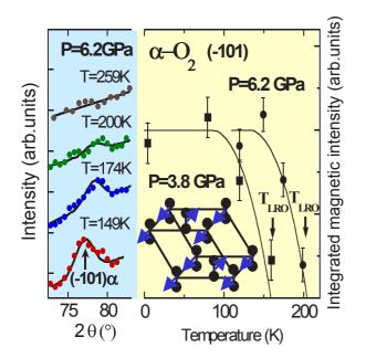
Figure 2 Left: temperature evolution of the magnetic peak (10-1) measured in  $\alpha$ -O<sub>2</sub> at P=6.2 GPa. Right: integrated magnetic intensity of the (10-1) peak versus temperature at pressures of 3.8 GPa (squares) and 6.2 GPa (circles). In inset: magnetic structure of  $\alpha$ -O<sub>2</sub>.
