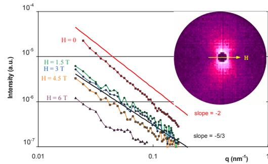
Figure 1. Magnetic SANS intensity from a  $\text{Pr}_{0.67}\text{Ca}_{0.33}\text{MnO}_3$  single crystal, for a set of increasing fields from 0 to 6 T after Zero Field Cooling to 4.2K. The two straight lines are power laws with exponents  $-2$  and  $-5/3$ . Inset: Typical PSANS spectrum showing the  $\sin^2\alpha$  contribution of magnetic scattering.
