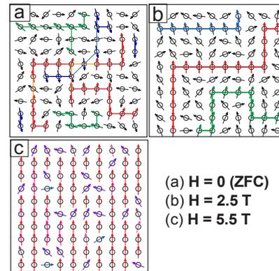
Figure 3. Schematics of the evolution of the filamentary phase with the applied field. From a disordered assembly of small filaments after the ZFC procedure, the applied field makes filaments with spins parallel to  $H$  grow, and shrinks the other ones. As the field continues to increase, the filaments percolate at 3.9T and then fade into the background when the difference in magnetization is too low to keep the carriers inside the filaments.
