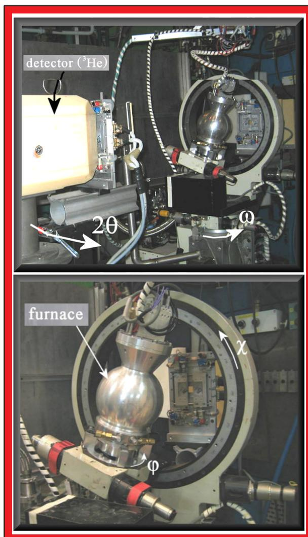
Figure 1 : Presentation of the furnace installed on the 4 circles 6T1 diffractometer
