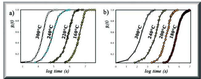
Figure 3 : Recrystallization kinetics of copper for two deformation rate a)  $\epsilon=1.27$ . b)  $\epsilon=2.84$ .
