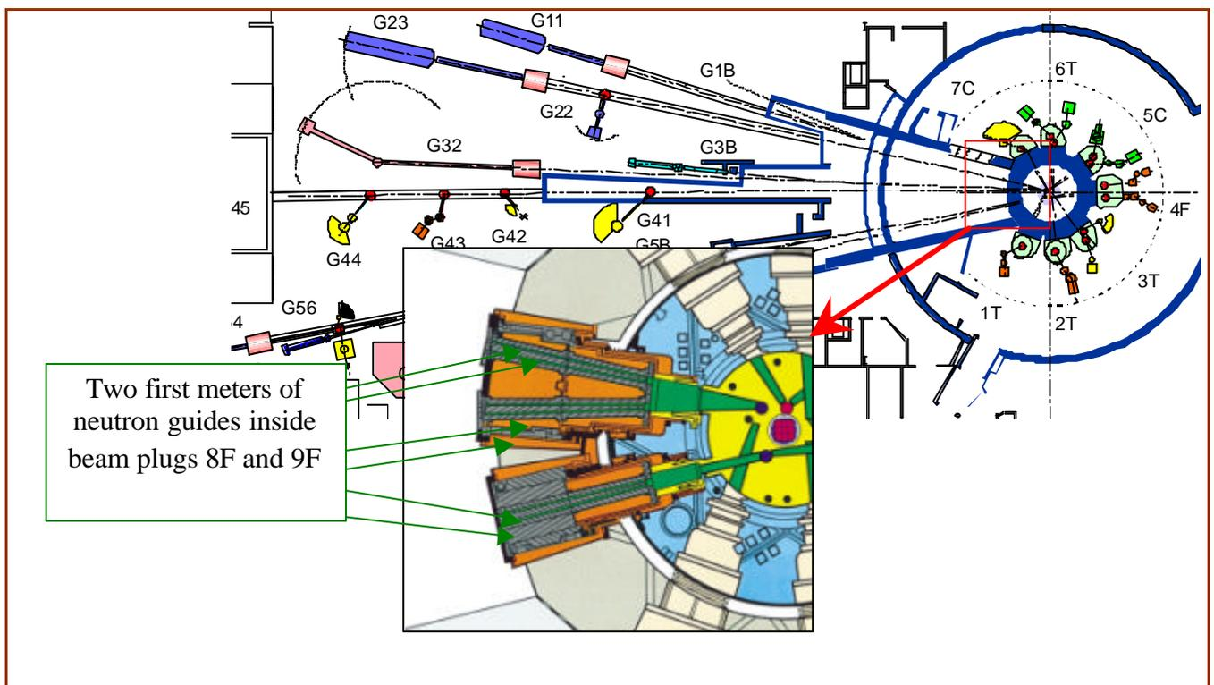
Figure. General layout of the guides elements within the 8F and 9F beam plugs.
