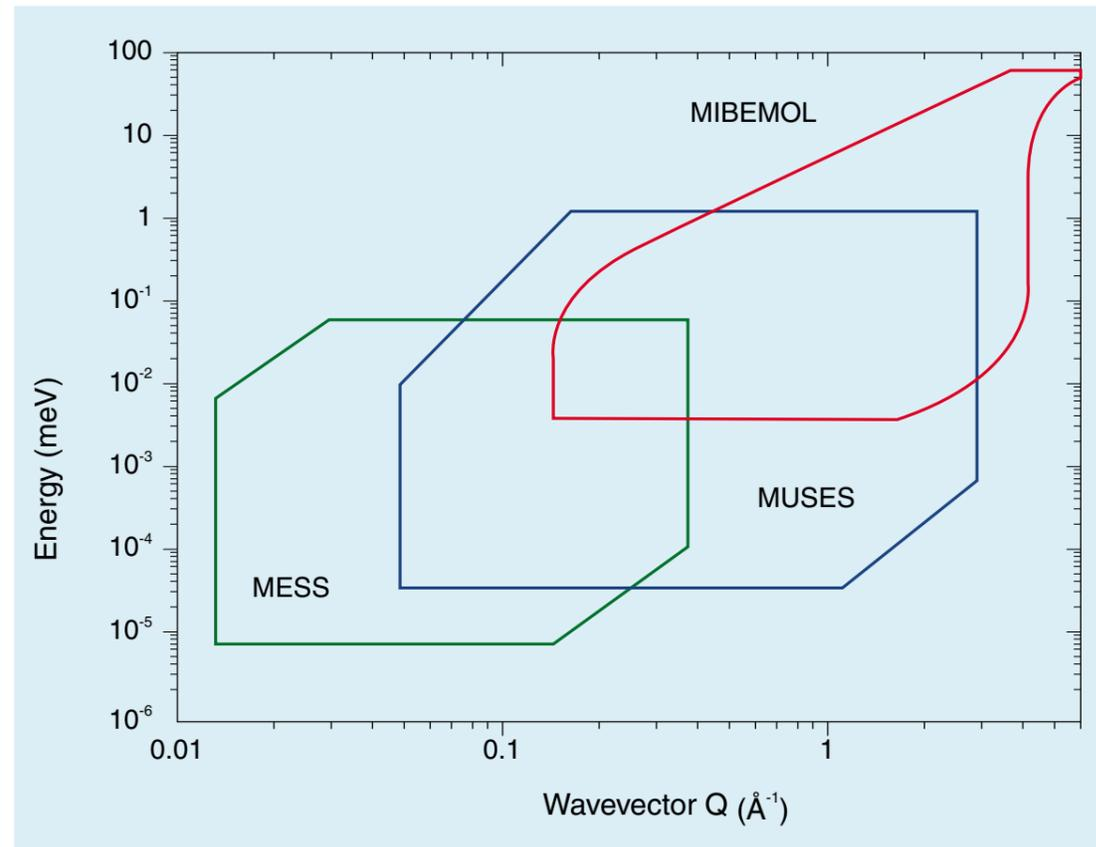
*Energy - wavevector domain cover by each spectrometer*
